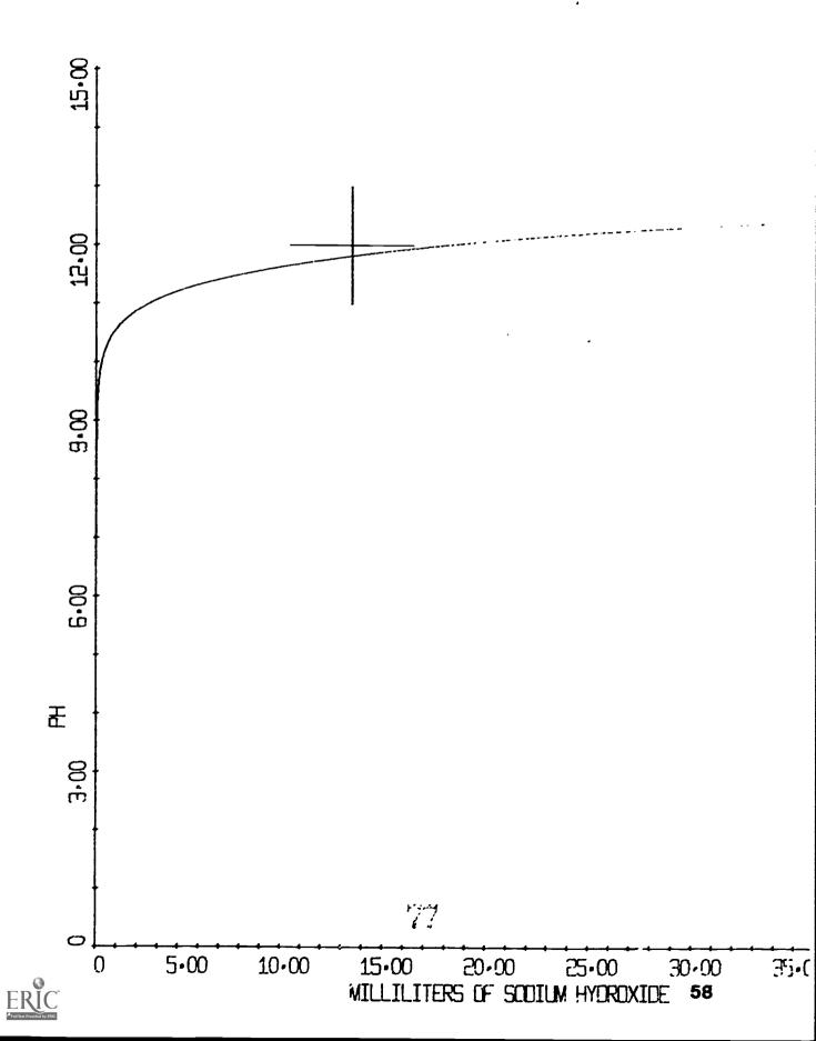
searching process at the beginning of the calculations, when the program is looping until  $V_{MOH}$  becomes positive, the pH increment is too large. It is possible for an overshoot of almost 0.5 pH units to occur. This is of no consequence for a weak acid, where the titration curve begins with a rather steep slope. The simple remedy for this problem (if you consider it to be a problem) is to reduce the pH increment to some smaller value by modifying one statement in the program.
